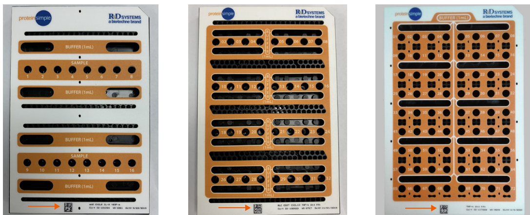
Figure 3-3: Cartridge ID barcodes: 16x4 (left), 32x4 and 32x8 (middle), 72x1 (right). The 48-Digoxigenin cartridge's barcode (not shown) is at the top of the cartridge.
