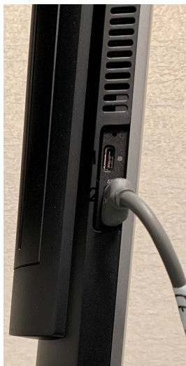
Figure 1-6: Monitor stand side view showing Barcode scanner and optional LAN (adapter not shown) interconnections.
