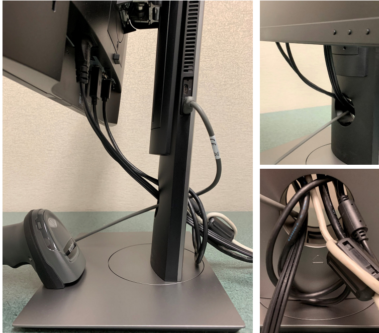
Figure 1-7: Clockwise: Side, lower front, lower rear (showing both monitor cables from the PC coming out the back looped once around the Ella cables and then out the front to monitor).
