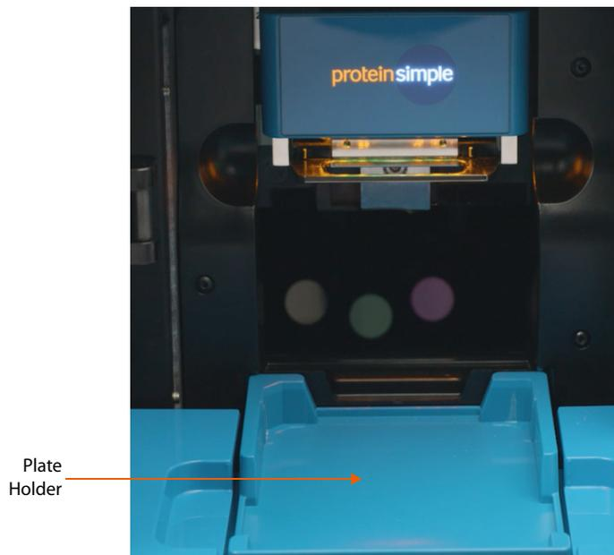
Sample plates should be inserted into the plate holder so that the A1 well position is aligned with the upper left corner of the tray.
